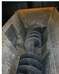
View inside hopper: Bi-directional, variable speed 36" (915mm) diameter auger with hard-faced flights for extended life.
