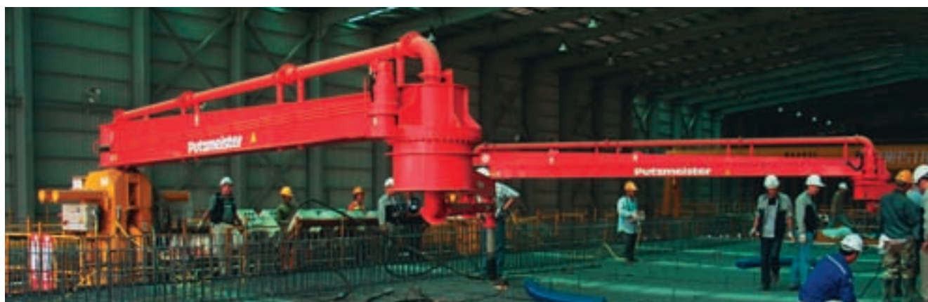
RV 16 rotary distributor in use in the production of bridge sections
