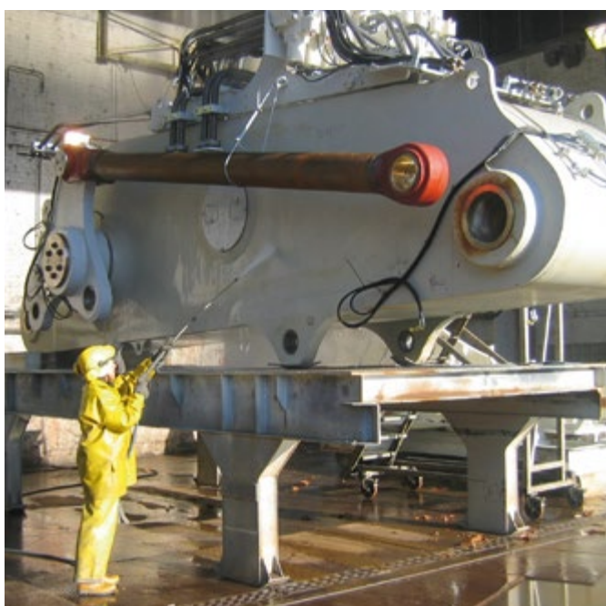
Preparing installations for paint removal
